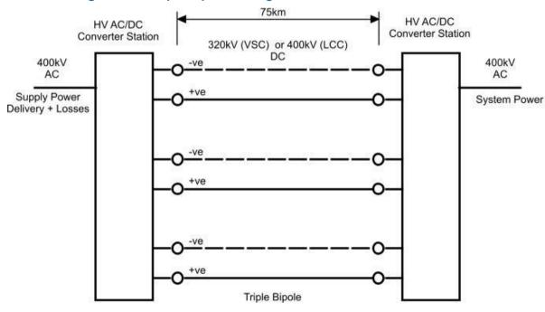
Each bipole would be buried beneath the seabed where possible to a typical depth of 1.0m as indicated in Figure 54. When installing more than one bipole it is good practice to separate each bipole by a comfortable distance of several hundred metres. This allows the cables to be buried safely without the installation vessel risking damage to a previously
