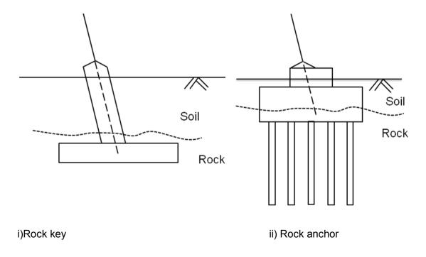
Even when the ground material is good or moderate it may not be convenient or practical to install a standard footing. In many instances, it is quicker or easier to install other types of foundation such as pile or caisson. With suitable designs in place, this option may be employed at the discretion of the contractor and may even be applied instead of rock
