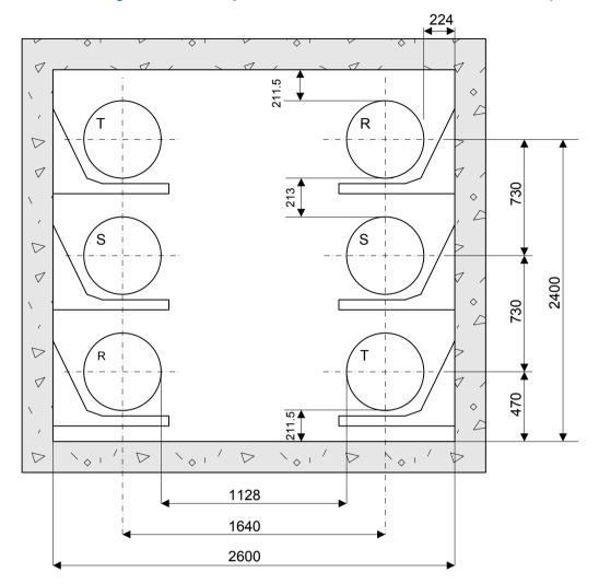
Figure 64 – Example of GIL double circuit in vertical-sided (surface) tunnel
