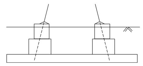
Pile and caisson type foundations are particularly useful for installation on steeply sloping ground where landslides and slope failures may occur, as the founding depth can be such that it extends below the failure slip plane. An example of a pile or caisson foundation installation in unstable sloping ground is shown in Figure 14.
