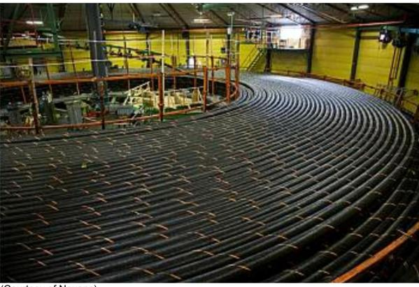
Figure 51 – Subsea cable on factory turntable.
