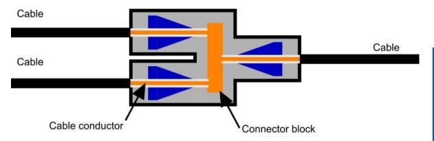
The Y-branch joint would allow the number of cables to be doubled locally for example to cross deep beneath a river or road or to pass through an area of constricted width.
