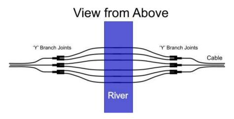
If a single cable conductor's load is shared equally between two equally sized conductors the load on each conductor is halved and the total heat loss is also halved. This allows the cables to be buried significantly deeper, or the phase cables to be placed closer together, before the temperature of any conductor rises to an unacceptable level.
