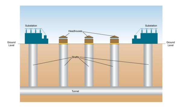
Figure 66 - Cable tunnel outline schematic
