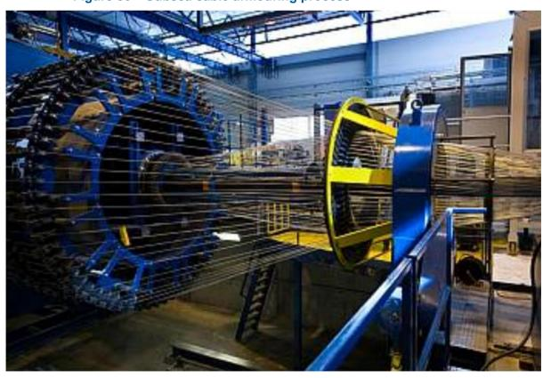
Figure 50 - Subsea cable armouring process
