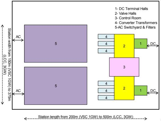
Converter transformers are heavy items of equipment (often over 100 tonnes each) requiring appropriate foundations and oil bund, interception and storage areas.
