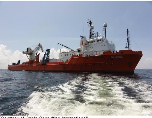
Figure 57 – Subsea cable repair vessel (DP Reel)
