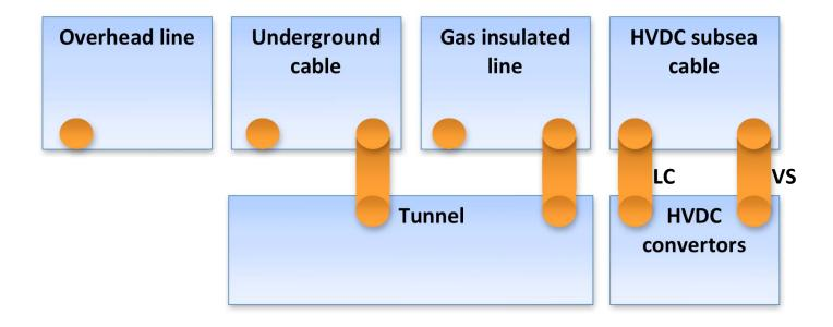
Figure 1 – The seven sets of transmission technology cost assessments
