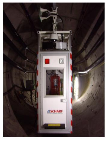
Figure 70 – Tunnel vehicle suspended from monorail
