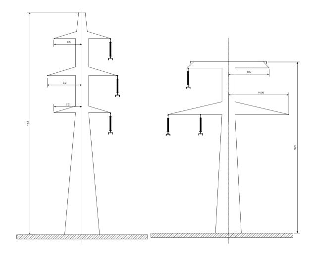
For 400kV, towers are usually spaced around 350 to 450 metres apart and provide ground clearance of at least 7.5 metres (recently increased to 8.1m to meet European Union requirements) in all weather conditions. Higher clearances usually apply if the route crosses motorways, navigable waterways or railways.
