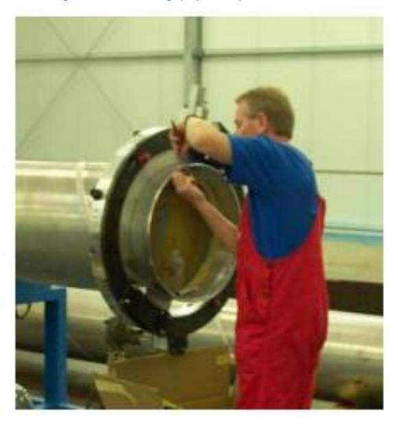
Figure 61 – GIL weld edge preparation prior to connection
