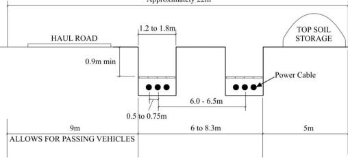
Figure 32 – Double circuit two cables per phase – swathe cross-section
