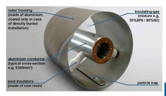
Figure 60 - Short section of gas insulated line, by Siemens
